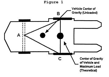
Notes: 1. When the vehicle is loaded, the combined center of gravity shifts toward line B-C. Theoretically, the maximum load will result in the center of gravity at the line B-C. In actual practice, the combined center of gravity should never be at line B-C. 2. The addition of additional counterweight will cause the truck center of gravity to shift toward point A and result in a truck that is less stable laterally.
